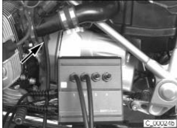
Throttle Synchronization Test
